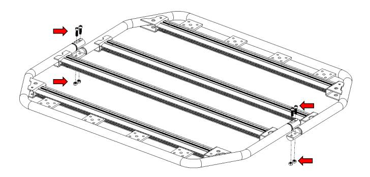
Place the sections so the coupling joint matches each other. Secure each side using (2) 5/16" allen socket bolts and (2) 5/16" hex nuts.
