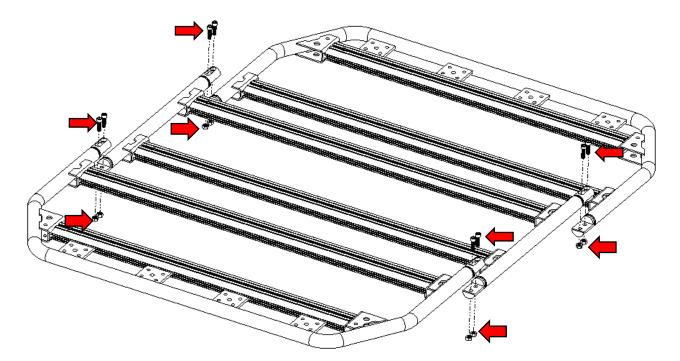
If you want to extend the rack use a connecting center (sold separately). Place the sections so the coupling joint matches each other. Secure each section using (2) 5/16" allen socket bolts and (2) 5/16" hex nuts.
